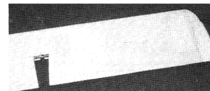
14. Elevators and stab taped together ready for MonoKote covering.
