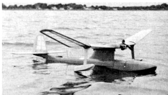
Years of research and development went into development of a design with excellent ROW characteristics. Model weighs 64 oz., gets off in 50 ft.
