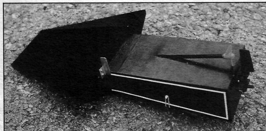
Underside view showing drive and rudder system. Note turn fin on one sponson. All photos: Author.
