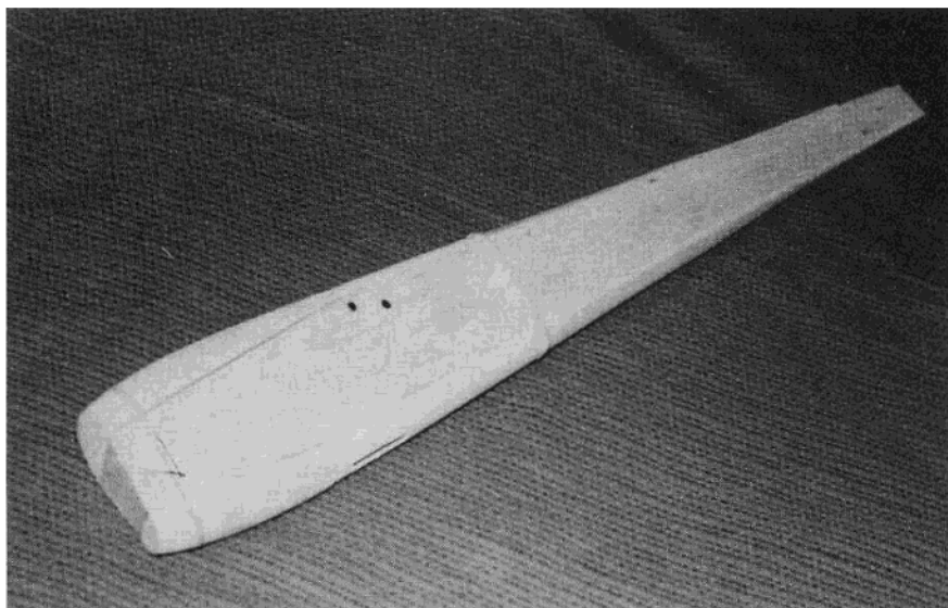
All fuselage top and bottom blocks and sheeting in place, and rough shaped; ready for nose block installation, shaping, and rough sanding.
