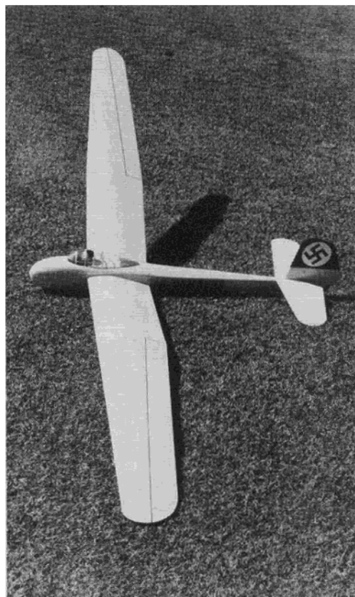
Completed model ready for flight. Trim tape and MonoKote trim sheet used for detail.
