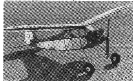
above: The Satyr has a delicate look because thinner hardwoods are used, yet this aircraft is very strong.
