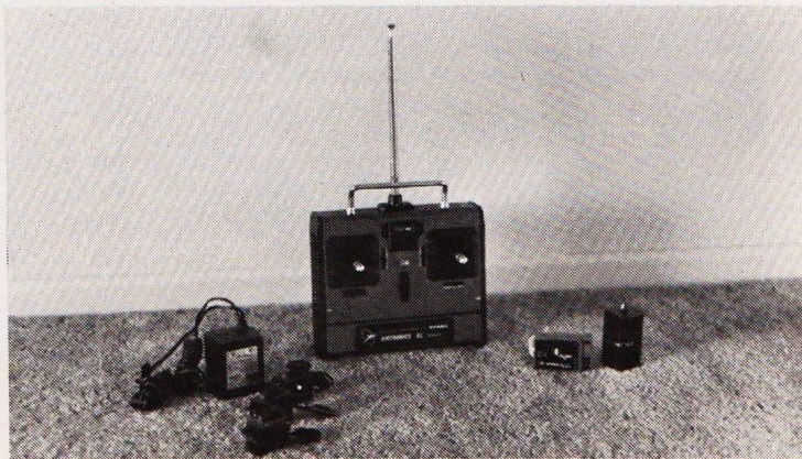
Radio installed in Sagitta was Airtronics XL series 3-channel; 94421 servos were also used and they are small and powerful.
