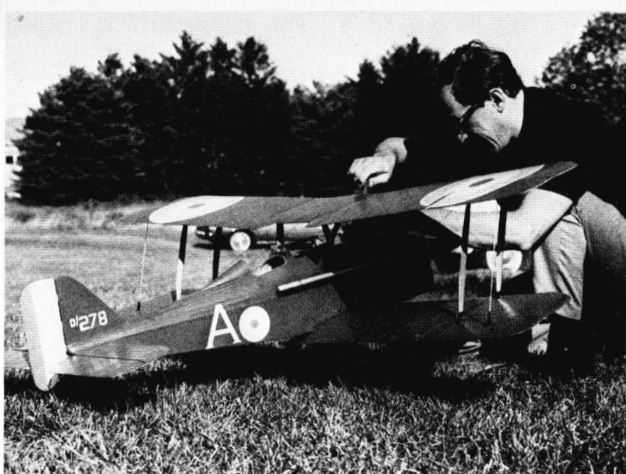
Important that flying wires be correctly bent and properly installed as these are all that retain the wings.
