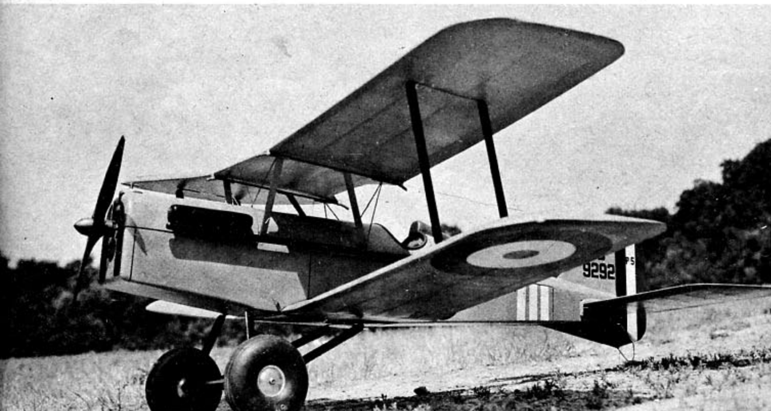
Adequate power for the SE-5 is developed by the ED 2.46 Diesel, approximately a .15 by U. S. displacement. Remove lower wing for access to radio.
