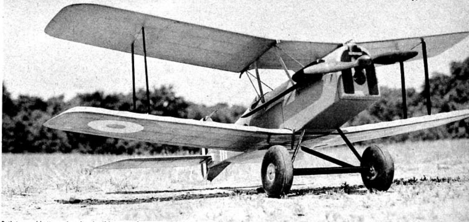
Both top and bottom wings knock off in event of a crash or, shall we say, hard landing? Excepting airwheels and stabilizer area, everything is to scale.
