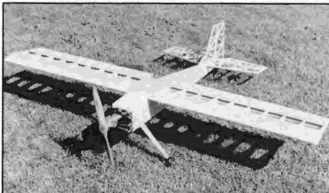
As can easily be seen here, this is a very simple airframe. Note the Saito 300 engine being used to power this model.
