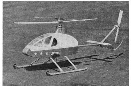
Author's RS with home-built collective pitch head.
