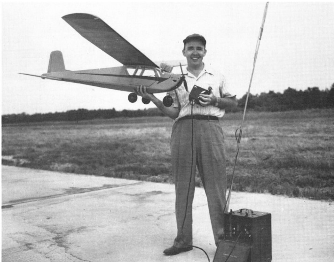
A happy Walt Good after his 1952 R/C duration record flight of 40 minutes, 28 seconds, at Andrews Air Force Base, near Washington, D.C. The model is his 6-foot Rudder Bug, with a Forster .29 ignition engine. Transmitter control box is in his left hand. Radio is described in text.
