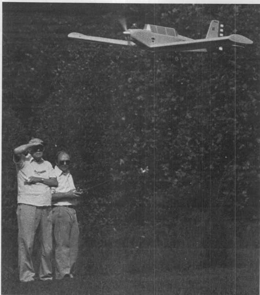
With test pilot Don Srull at the controls, the Rookie II makes a low-n-slow pass for photographer Tom Schmitt. Tip plates increase aileron effectiveness at low speeds.
