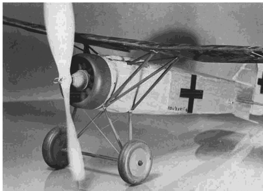
Wing and cabane strut layout shown in detail here, also wire axle springing. Wheels were heat-formed over wooden master.
