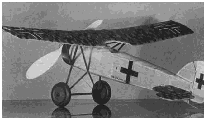
Camouflage on upper surfaces shows well here. Author tells how he did it, in the text. Note bond paper decking and side cowl fairings.
