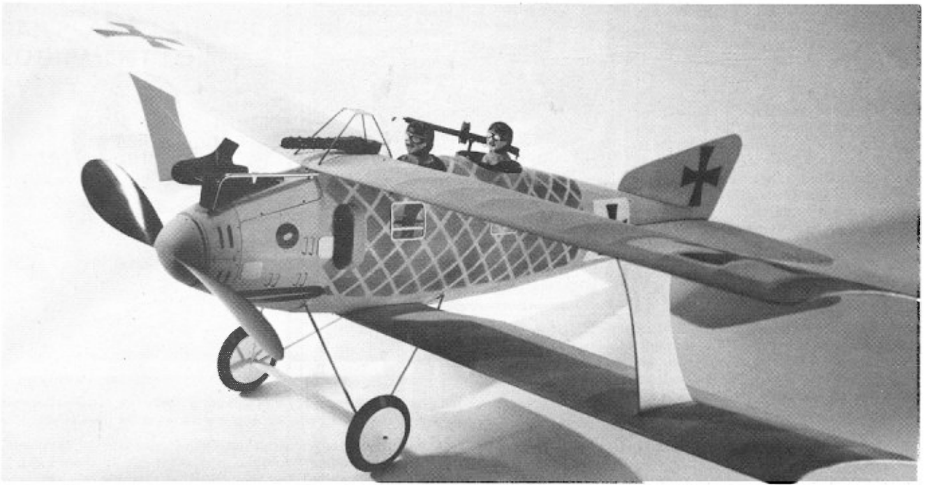
There's a lot to recommend the Walfisch as a modelling subject; longer than usual nose moment, no canopies, widespread gear, and little rigging.
