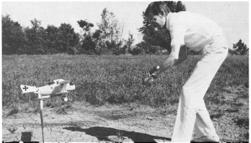
Packing in the winds. Dave used two loops of \frac{3}{16} by 30 inch long rubber in the Walfisch . Braid the motor about 100 turns, then crank in 300 turns for initial trim flights. Maximum turns run about 1400.
