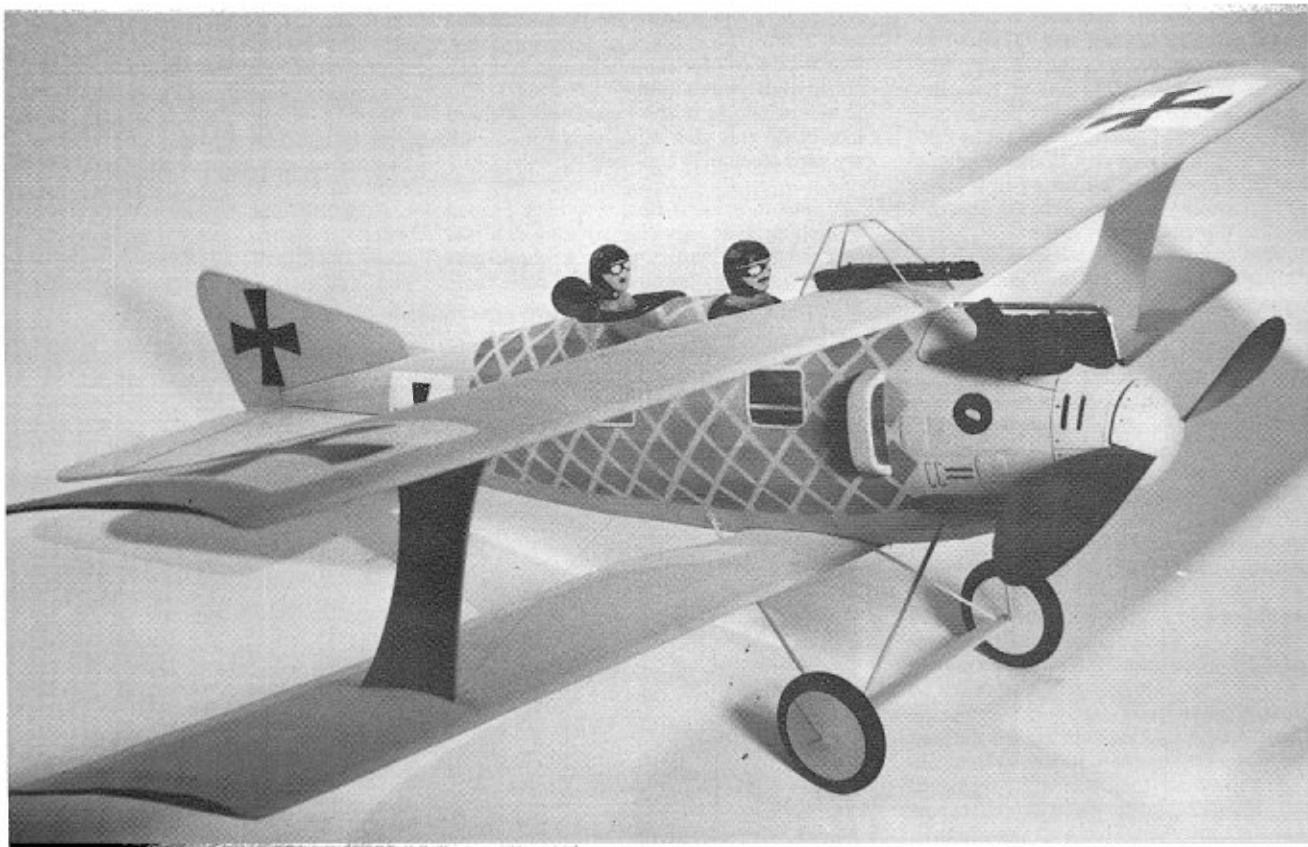
The fish scale finish is not as difficult as it might seem. It was created using a graph paper mask. Darker color is Pactra Insignia Blue.
