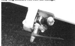
Top view of nacelle. Half-cowl looks good in flight but gives easy access to engine.
