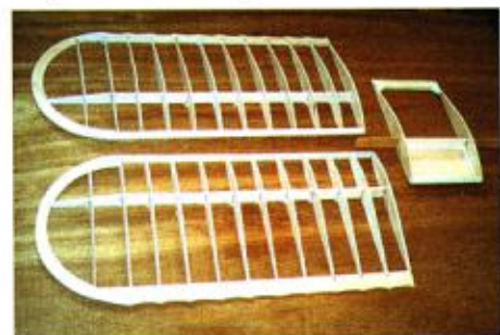
Basic 3-piece wing construction before joining. Note scalloped TE.
