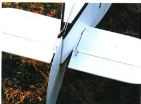
Tail assembly reveals tiny pushrod and control surface linkages.
