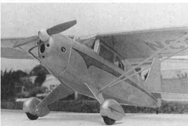
Note small wire protruding from cowl bottom for glow plug clip.
