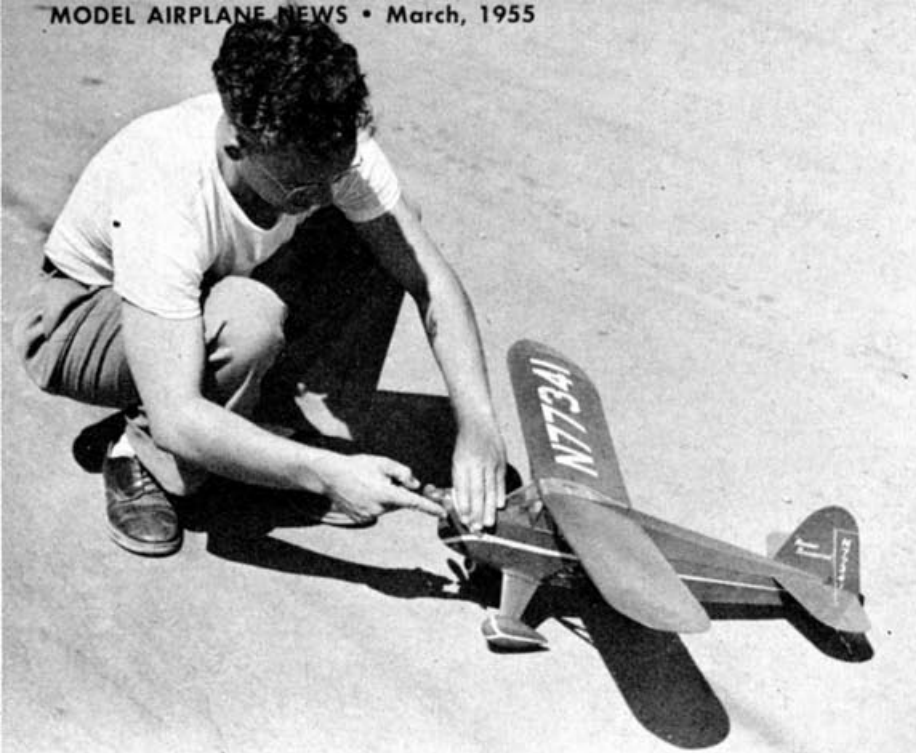
Flipping the prop on his McCoy .049 Diesel, Walt prepares to take off the original model. The small amount of right thrust, plus wash-in both wing panels, provides left climb circles, right in glide.
