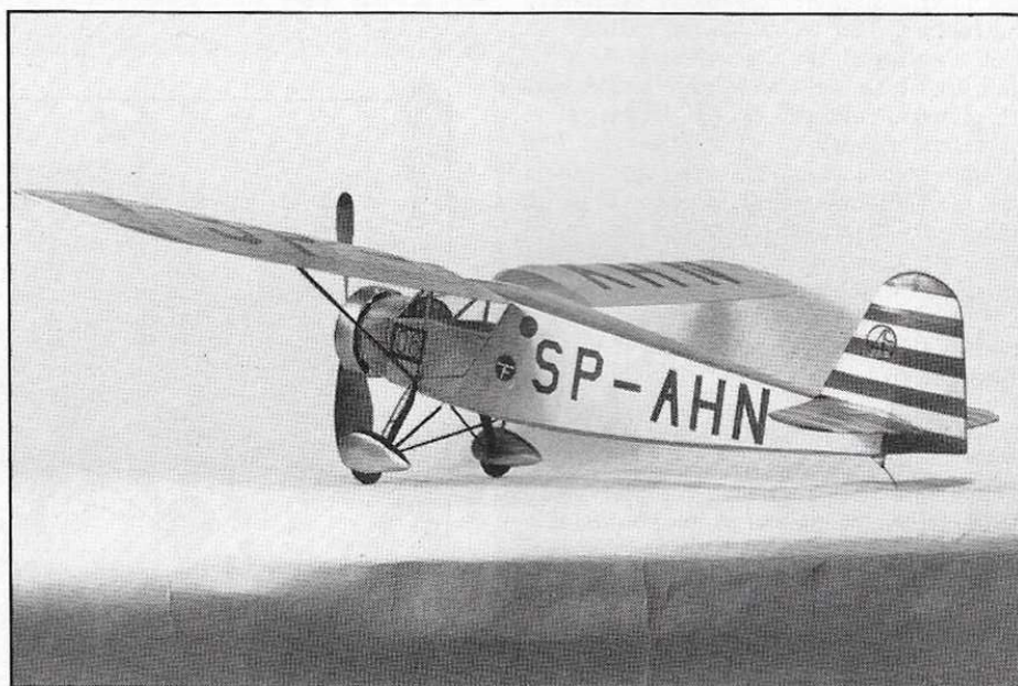
Fuselage lettering can be cut from good quality black tissue or stenciled and sprayed. Original model was test flown on Peck 9 inch plastic prop and 1/8" rubber. Author has logged consistent one minute flights.
