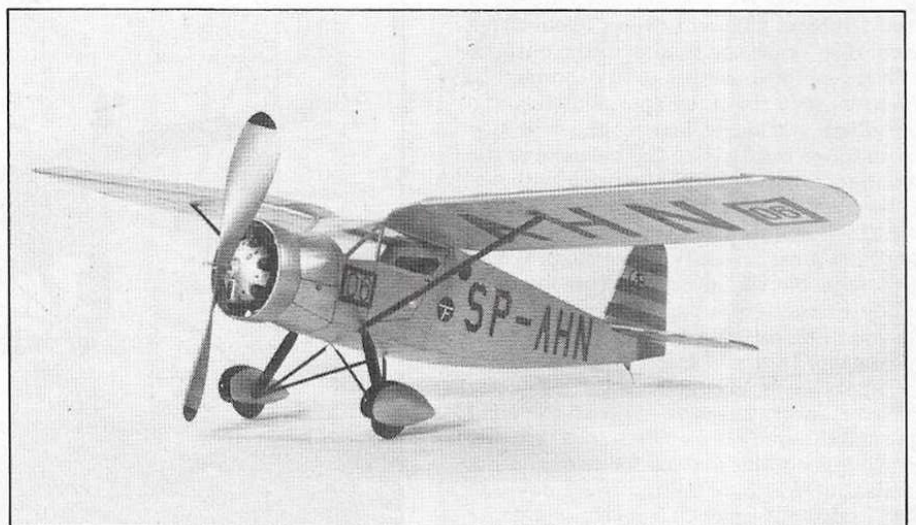
The forerunner of today's STOL aircraft, the R.W.D.-6 is relatively simple and has pleasing lines. Wings are aligned with aluminum tubing and alignment pins. Williams Brothers engine cylinders add detail.
