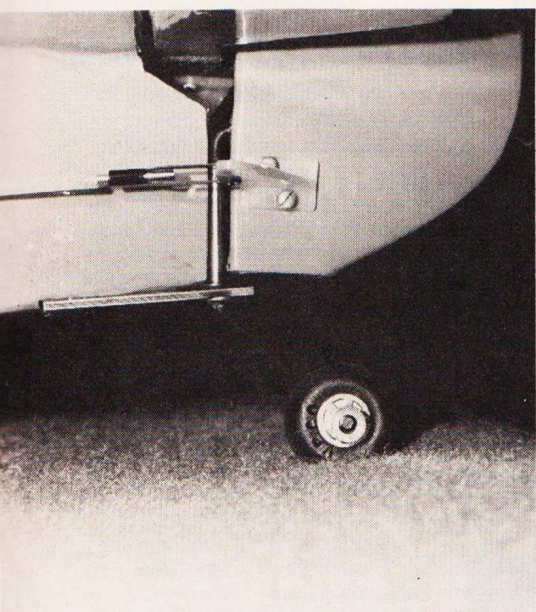
Tail wheel and rudder use simple coupling hook-up.
