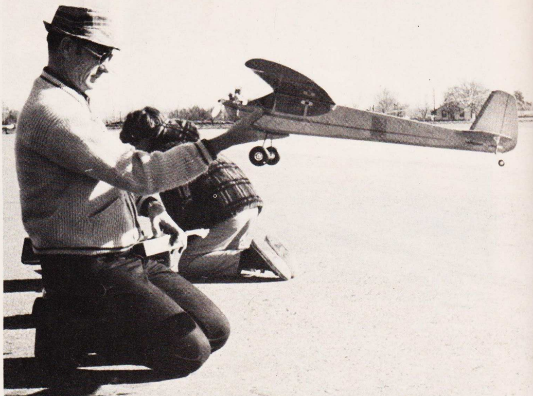
Bill Shelby, author's flight instructor, checks wing alignment as part of the pre-flight program.
