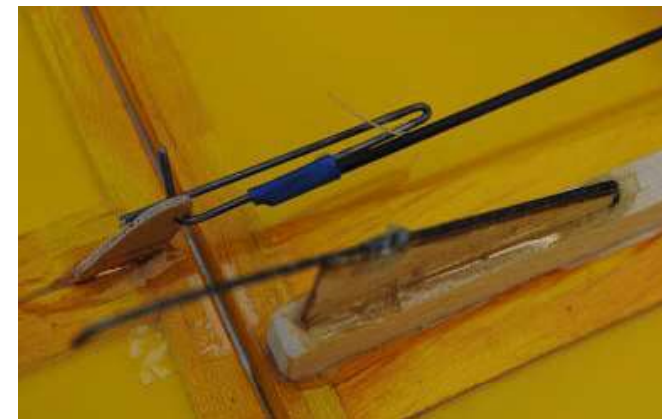
Wire end on .050 carbon fiber push rod held with heat shrink tubing and a drop of CA. Won't slip, but can be adjusted. Ply and wire tail skid.
