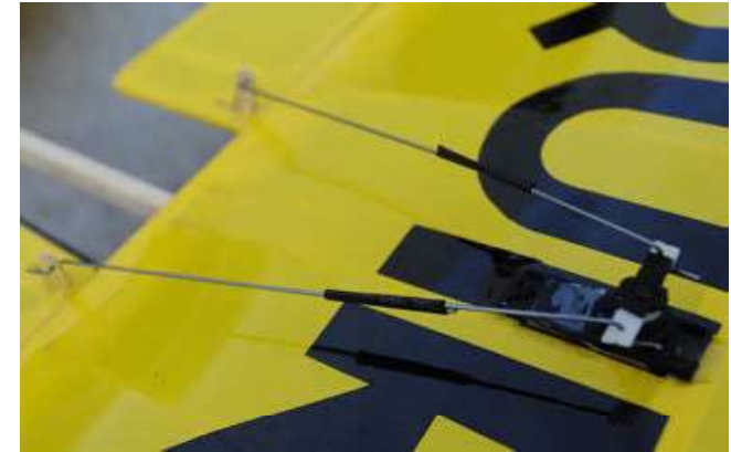
Aileron pushrods are two pieces overlapping in heatshrink tubing.
