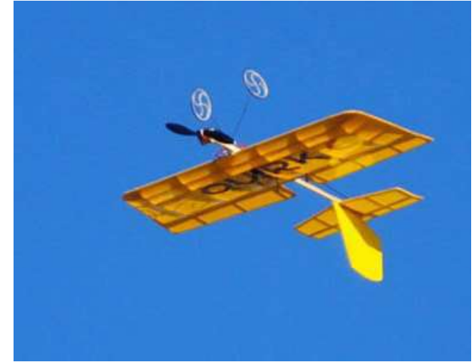
Quirk-e gliding gently, lazily, inverted. Arm your ESC's brake for best glide.
