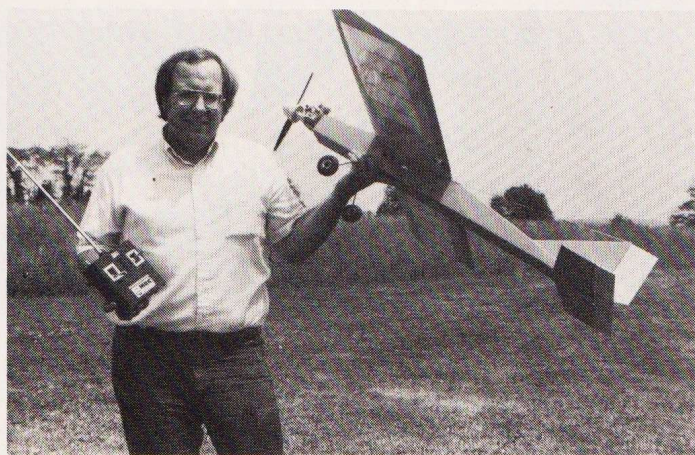
This view from the rear shows the constant width fuselage to good effect. It is strong and easy to build. Bob gives us a look at the undersides (right). Strong landing gear mounts for rough fields. Generous rudder.
