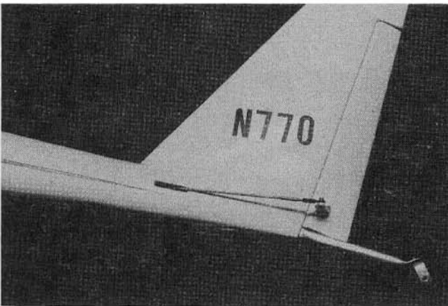
Photo shows rudder linkage and tail wheel detail. Note ball link is used on rudder horn for angled rudder.
