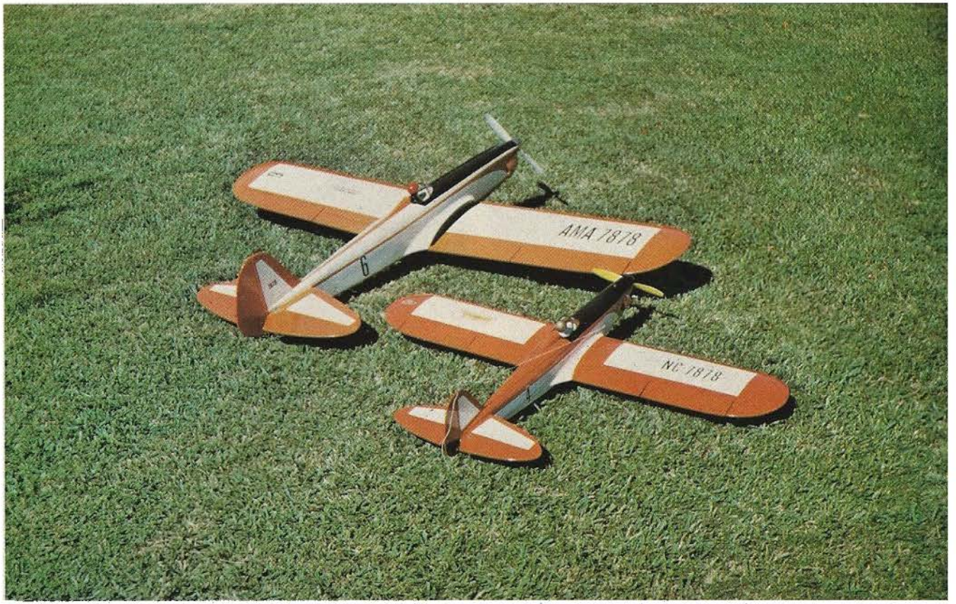
Two of the author's stable of Puffin's. The larger version is the one presented in this article. Designed to fly at weights varying from 6 to 8½ lbs.
