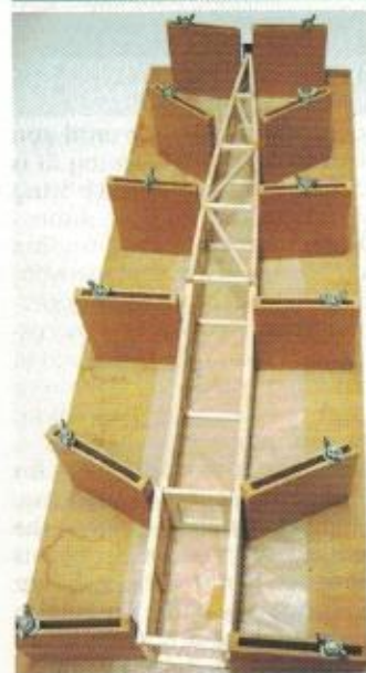
Above: Fuselage side frames are jigged and joined with cross members
