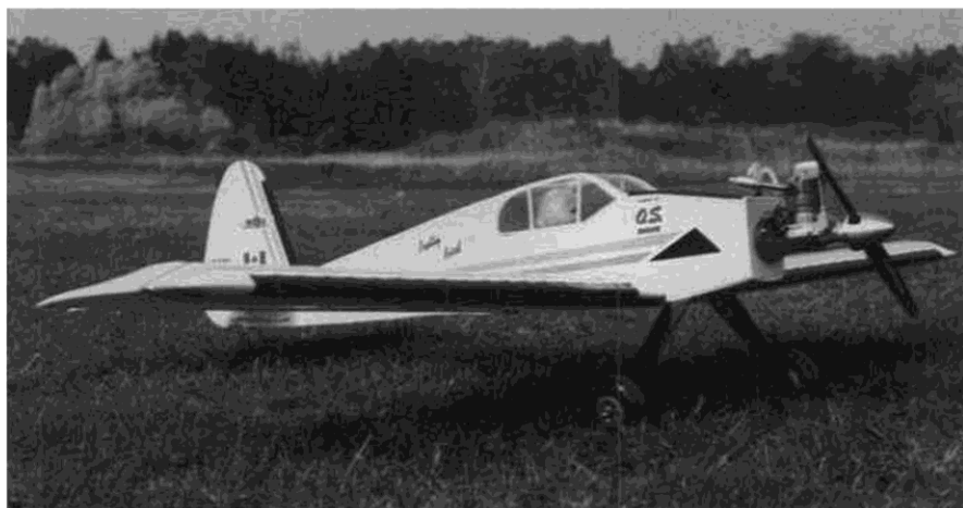
Uncowled engine keeps things simple. Model is shown here with the original fiberglass landing gear, which was a bit too flimsy and was later replaced by the wire gear shown on the plan.
