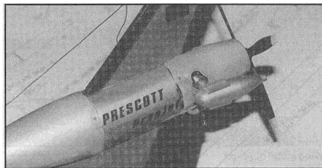
Elevator and rudder control horns. Note the pull-pull cables for rudder control.
