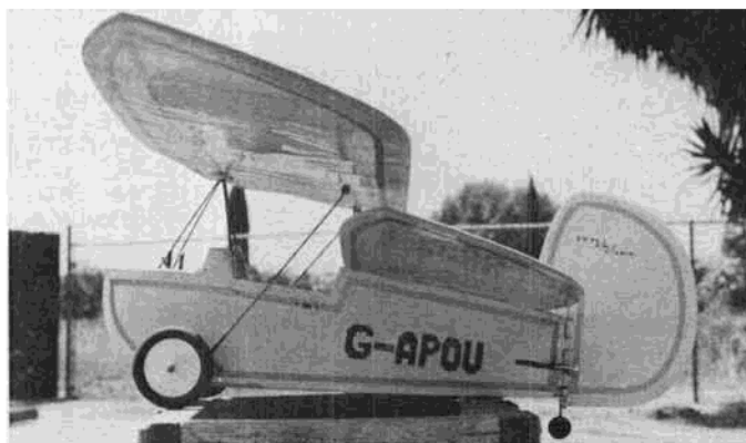
Side view of the Flooing Fly . . . er, Fleeing Floo . . . you know! Elevator pushrod clearly seen here. Darned unusual aircraft!
