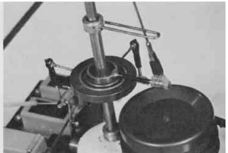
Swashplate control rod to steering paddle and anti-rotation yoke.
