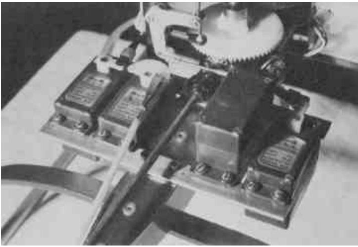
One of author's prototypes showing World Engine's S-4 servos mounted on 1/8" x 1/2" aluminum servo rails. Bob Depew photo.
