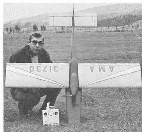
Author holds a much-flown Platypus. Note large stabilizer to compensate for wide bow area and neatly cowled engine.
