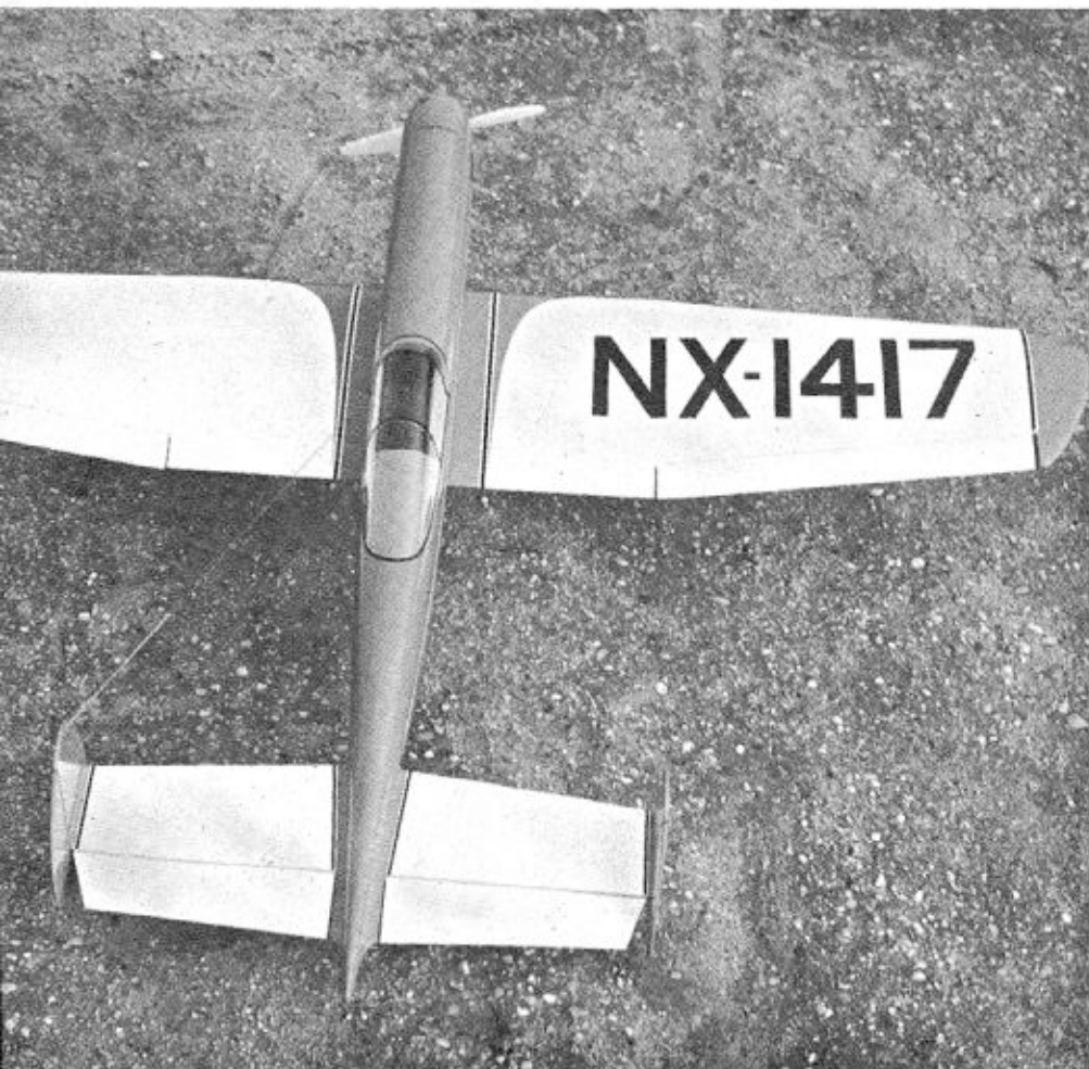
Hobbyoxy balloon molded fiberglass cowling. The advantages include great strength with a thin wall for greater air cooling. Make balsa form.
