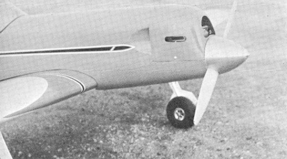
Hobbyoxy balloon molded fiberglass cowling. The advantages include great strength with a thin wall for greater air cooling. Make balsa form.
