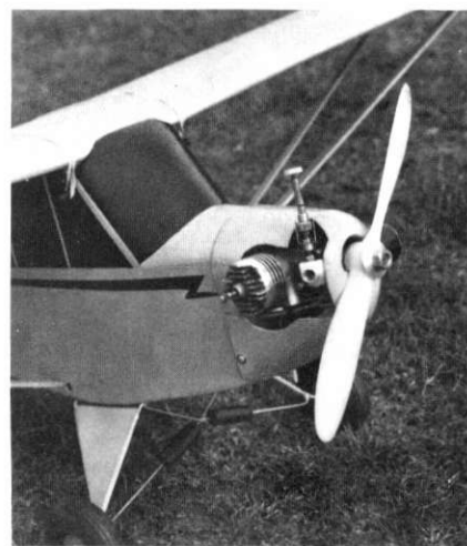
Below left to right: basic fuselage showing tank installation and built up formers; undercarriage retained by nylon saddle clamps, note balsa shock absorbers; stripwood planking for top deck; cowling made from 1/32in ply wrapped over balsa block hollowed out.
