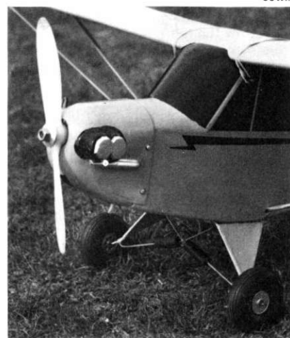
Below left: the Cub's front end, view showing Enya 15, don't forget you will need to fit a silencer. Below right: the dummy engine, note small screws retaining cowl.
