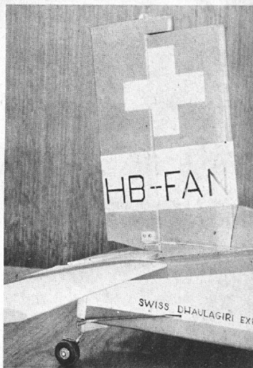
Tail unit of Pilatus Porter; shown are push rods for moving rudder and tailwheel.
