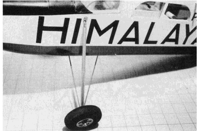
The aluminum tubing was slipped on, and eye lug soldered to the end of main leg.
