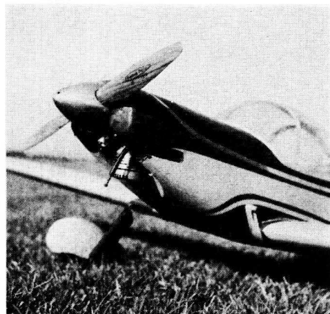
Inverted engine easiest to start. Don't prime into cylinder; just wet side of piston with fuel just before flipping prop.
