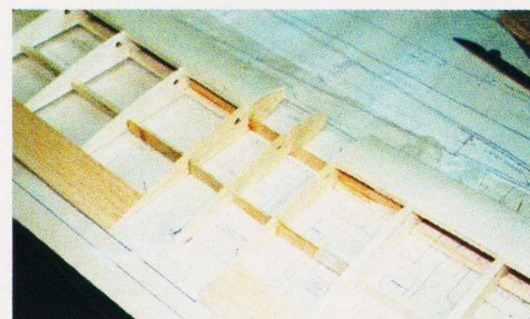
Joining the wings, pack up the tips 3/4" each side.
