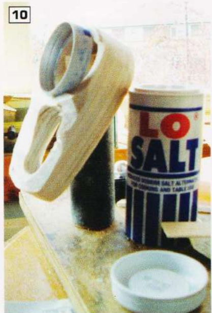
10 & 11: Noseblock fun..... cut the ring from salt dispenser and then put the lid back on. Salt dispenser then returned to kitchen ... without wife noticing! 12: Fully shaped nose block. 13, 14 & 15: Dummy cooling grill should be applied to both sides of fuselage. Strips of 1/16" balsa are chamfered and glued to card.
