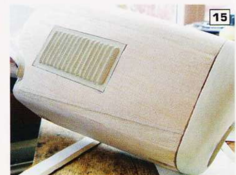
10 & 11: Noseblock fun..... cut the ring from salt dispenser and then put the lid back on. Salt dispenser then returned to kitchen ... without wife noticing! 12: Fully shaped nose block. 13, 14 & 15: Dummy cooling grill should be applied to both sides of fuselage. Strips of 1/16" balsa are chamfered and glued to card.
