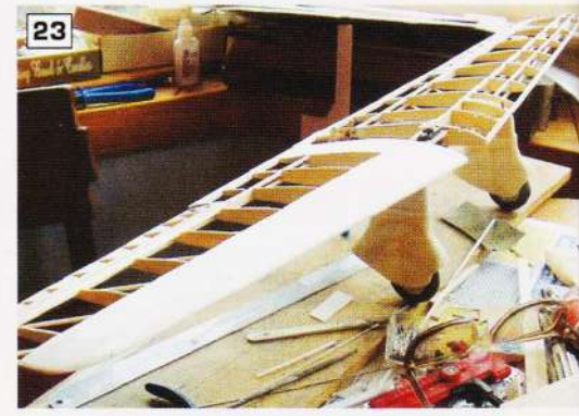
17 - 21: Wing/aileron structural detail. The Solartex hinges are 'trapped' by the 1/16" capping. Originally, carbon fibre torque rods were used to move the ailerons but, for the sake of buying one more servo (which are now much cheaper!) - go for the update. It's better and easier! Be sure to check that they work, and set up the operation with your tranny before covering. An inaccessible servo that turns out to be a duff ain't too amusing! 22: Laminated tips made from balsa strip that's been in the dishwasher! 23: 1/32" wing sheeting applied to top only while wing panel pinned to that jig - let me know if it does the job... (You can reply to the RC Groups build thread?)
