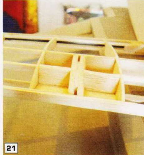
17 - 21: Wing/aileron structural detail. The Solartex hinges are 'trapped' by the 1/16" capping. Originally, carbon fibre torque rods were used to move the ailerons but, for the sake of buying one more servo (which are now much cheaper!) - go for the update. It's better and easier! Be sure to check that they work, and set up the operation with your tranny before covering. An inaccessible servo that turns out to be a duff ain't too amusing! 22: Laminated tips made from balsa strip that's been in the dishwasher! 23: 1/32" wing sheeting applied to top only while wing panel pinned to that jig - let me know if it does the job... (You can reply to the RC Groups build thread?)
