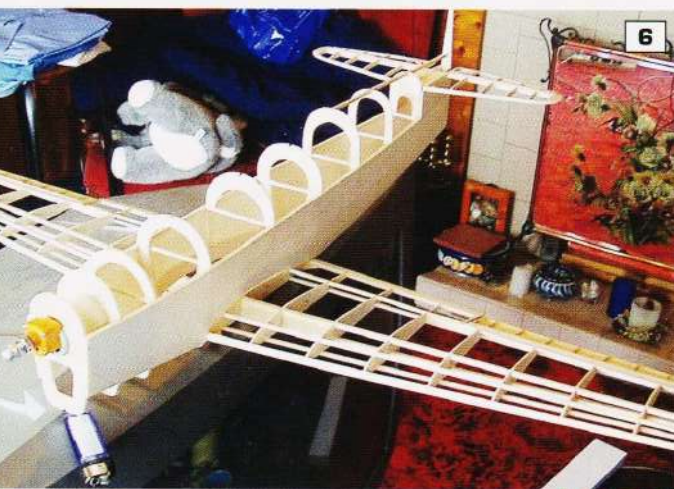
6: The basic airframe, assembled to see how it's all coming together.
