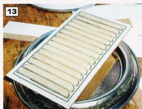
10 & 11: Noseblock fun..... cut the ring from salt dispenser and then put the lid back on. Salt dispenser then returned to kitchen ... without wife noticing! 12: Fully shaped nose block. 13, 14 & 15: Dummy cooling grill should be applied to both sides of fuselage. Strips of 1/16" balsa are chamfered and glued to card.
