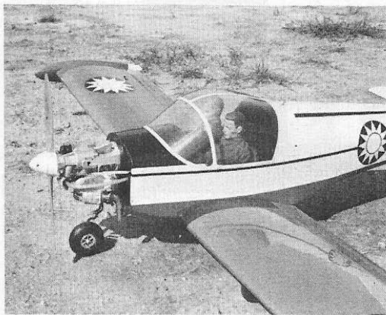
ABOVE: It is a fast and reasonably aerobatic flyer. Here, one can imagine a CAF cadet with instructor turning in on final approach for landing. LEFT: It is rather busy under the cowl. For nose weight a "D" cell nickel-cadmium battery for the glow plug is added. ST 46 provides the power even though the model weighs 6½ lb.
