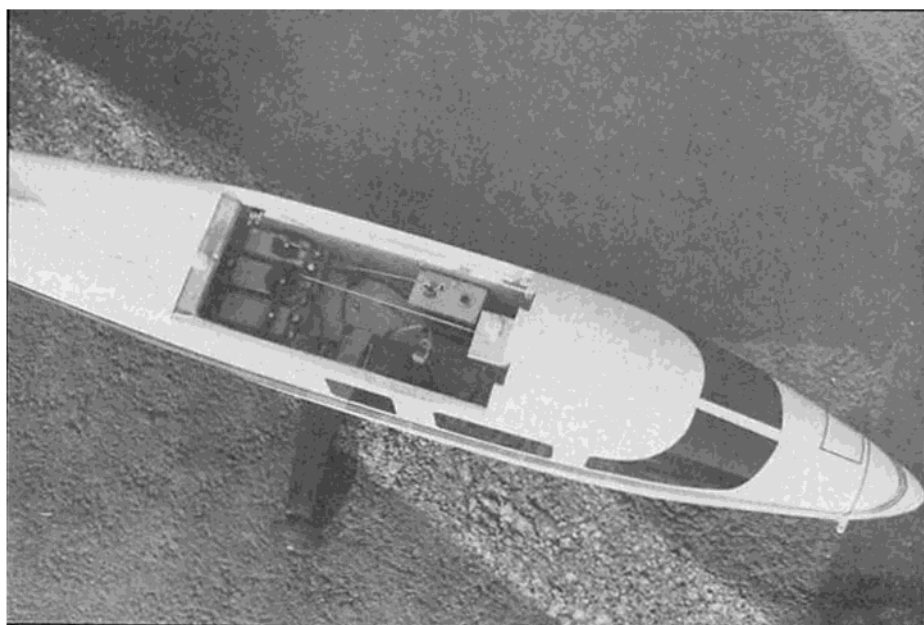
Plenty of room inside the Partenavia cabin. Note three-position speed control on left side of cabin and air exit slots at top of forward cabin block. Three S & O servos mounted at rear of cabin, aileron servo in wing.
