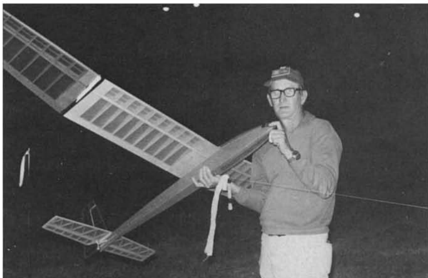
The author prepares for a night thermal flight. Note chemical lights at dihedral break.
