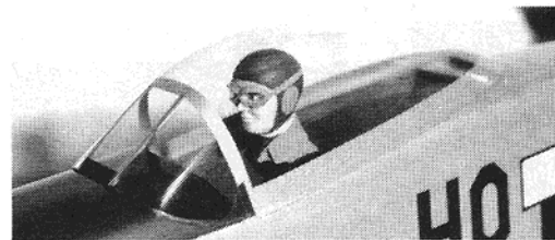
The P-51's 1/2-inch pilot is a trimmed down Williams Bros. figure, and the canopy is a 9-inch WW II canopy from Sig Mtg.
