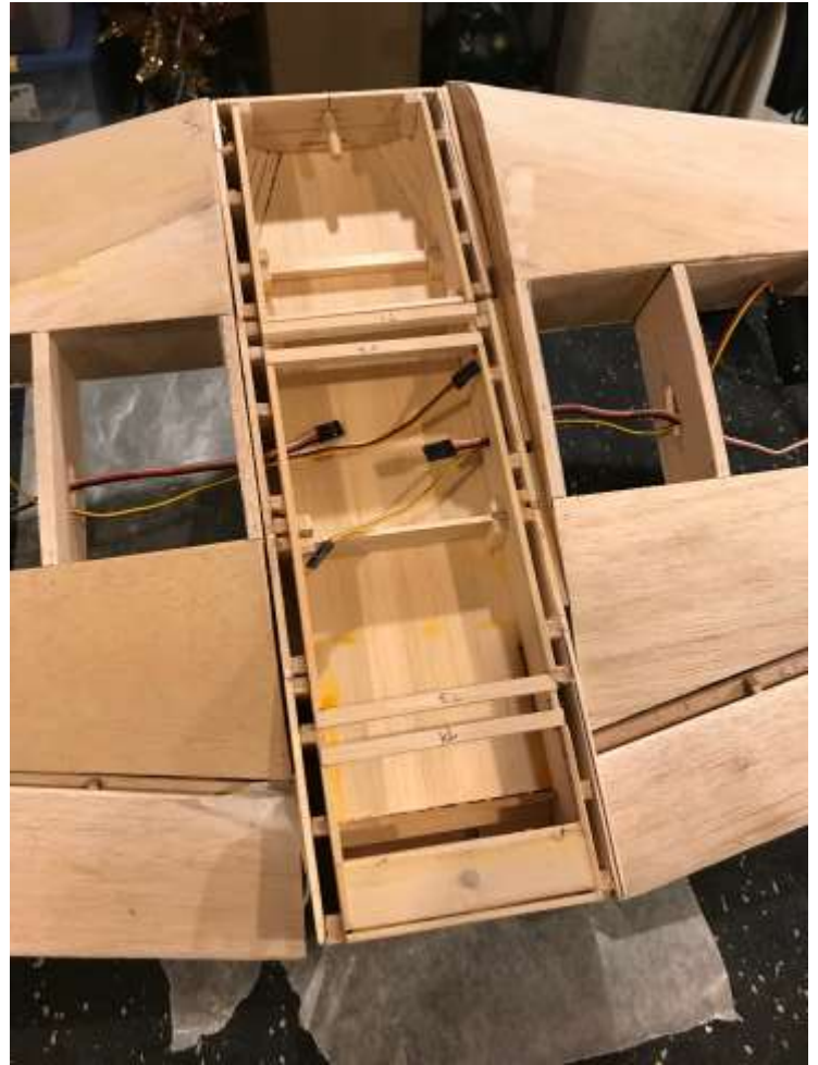
The iconic P-51B scoop has a 1/8" core and covered in balsa sheeting. Between the braces is a slit for the servo wires.
