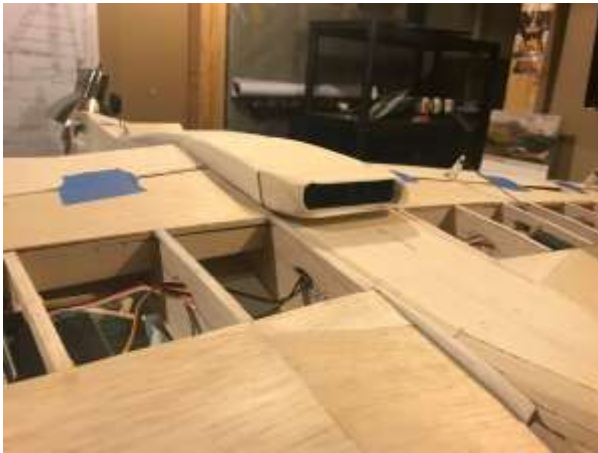
The iconic P-51B scoop has a 1/8" core and covered in balsa sheeting. Between the braces is a slit for the servo wires.
