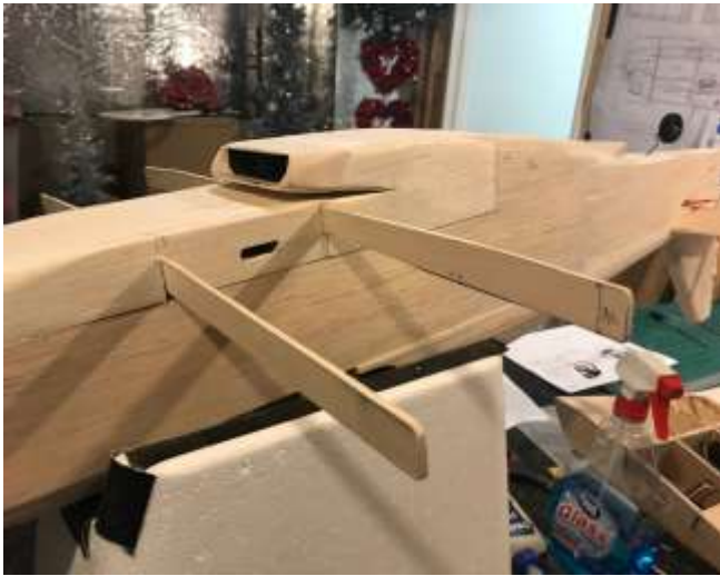
The iconic P-51B scoop has a 1/8" core and covered in balsa sheeting. Between the braces is a slit for the servo wires.
