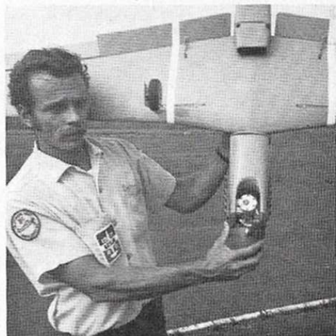
Above, Dave shows the inverted engine installation on his P-51. He plans to build another ship to add retracts for an even finer looking plane.
