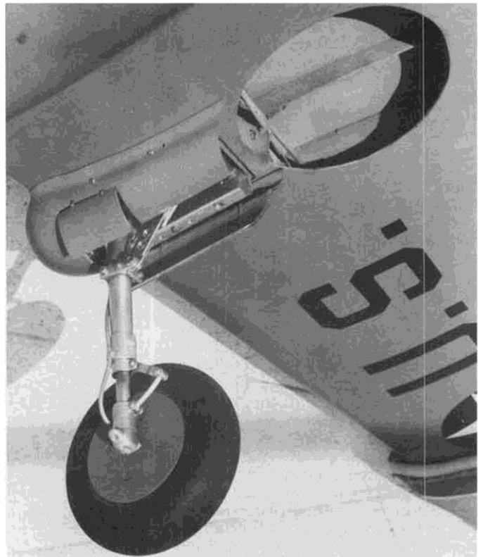
Above: Another flight shot by a passing spectator, using Art's camera with telephoto lens. A high 'G' pull-up, but gear stays in the well. The classic fighter aircraft. Right: The gear retracts 95 degrees and rotates 95 degrees. A complete follow-up article is coming, on how to build them. Brake lining is freon tubing.
