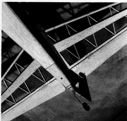
At left: End of an "Orion". Nylon tailwheel bracket, rudder horn, stab structure visible.
