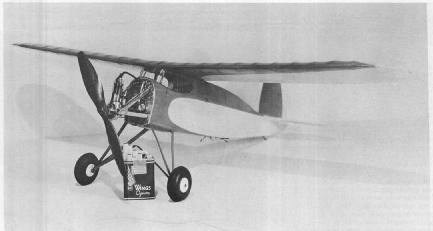
The 42-inch span model flew for the first time at what is now Edwards Air Force Base in California. Large prop kept plane low; Irwin speculates that smaller prop might have enabled model to fly at higher altitude. Replicas fly well with O.S. .10 FSR
