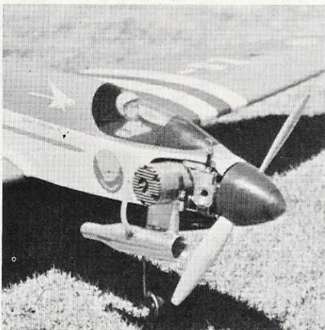
Webra Speed provides the motivation, while Silenciaire muffler keeps things legal and quiet.
