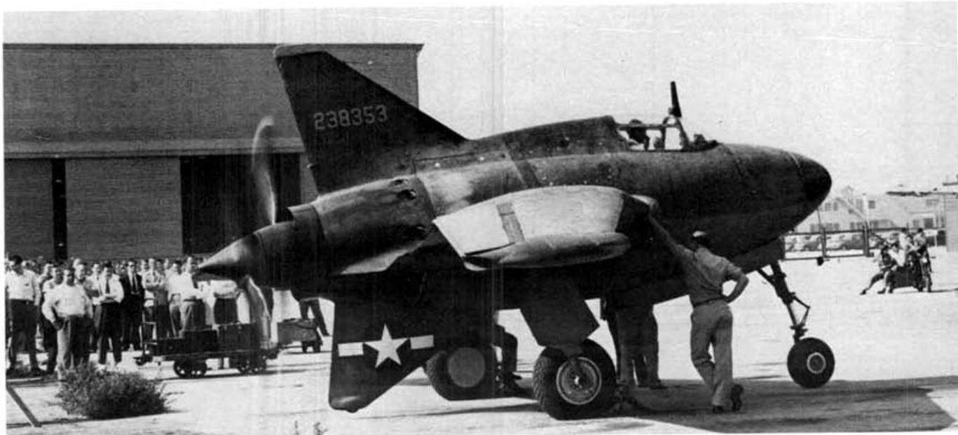
Northrop XP-56 No. 2 at Hawthorn Field. First welded all magnesium aircraft. Contracted for in 1941 by Air Corps. First flown on March 23, 1944 by Harry Crosby. Movies exist of this aircraft in flight. Pratt & Whitney R-2800-29 Double Wasp. Northrop photo.
