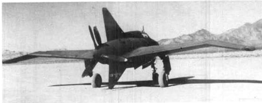
The XP-56 at Hooper's Dry Lake, in Nevada. Note closeness of lower fin to ground. Not much room to rotate for takeoff, but fin also protected props!
