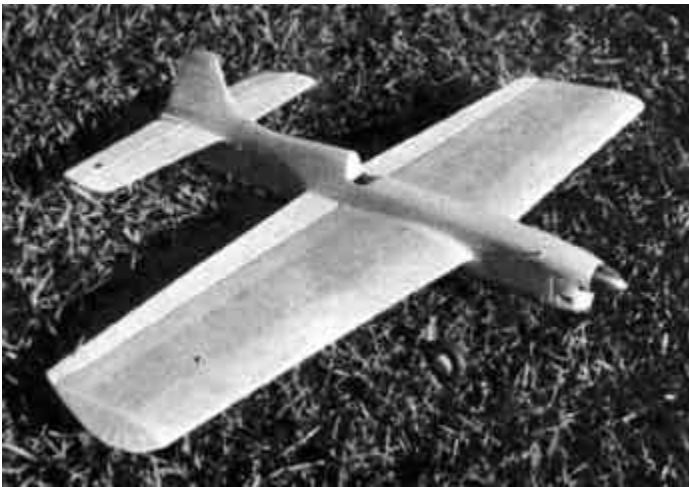
Finished model before painting. Covering has been water sanded preparatory to putting on the deep blue finish. With finish weight may hit 47 oz.
