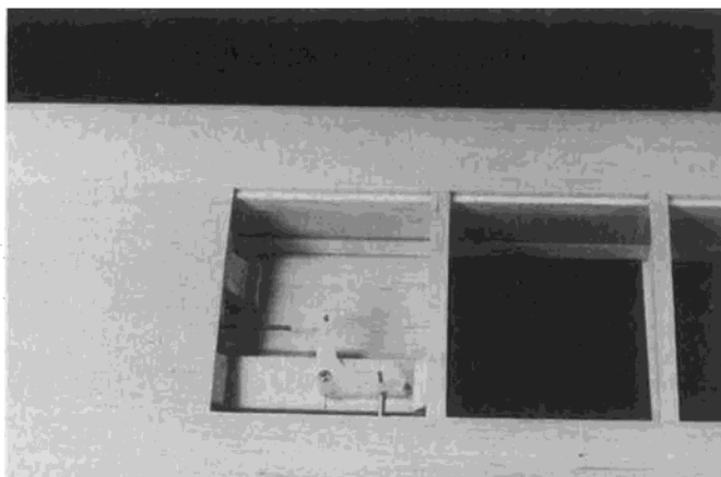
Aileron bellcrank. Note that link to horn is installed in middle hole.
